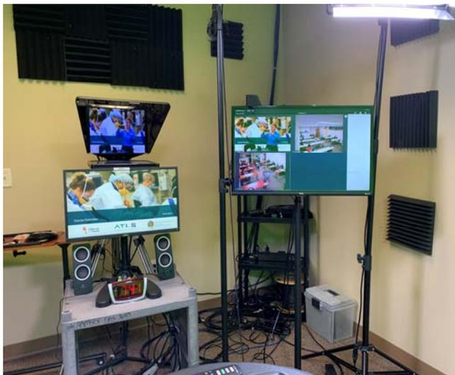
Note the monitor on the right. It shows a view of both conference rooms, as well as the slide being displayed. The instructor wears an earpiece that feeds audio from both rooms into their ear. The boom microphone overhead lets the instructor converse with the students in both rooms.
